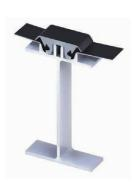
The attempt to form threads in the beam at the extrusion mill is not practical due to tolerances of the normal extrusion process. A screw will strip out the threads in the slot after one or two installations and will not develop maximum strength. No flange stiffeners are allowed due to manufacturing limitations. The gasket compression is the sole device for sealing the joint.
